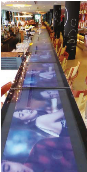
28 Samsung 40-inch table-top screens have been inserted into the customised aluminium framed tables of the Beast & Butterflies
