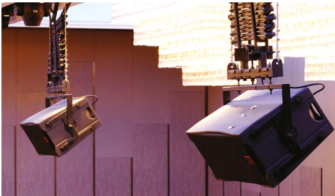
Sound reinforcement can be added courtesy of L-R Norton i1212W 3-way coaxial loudspeakers
