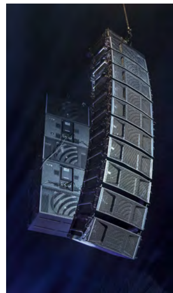
The main hangs consist of 10 Panther loudspeakers
