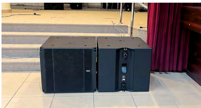
KROSS SUB 21 subwoofers have been installed in a 1:1 cardioid configuration
