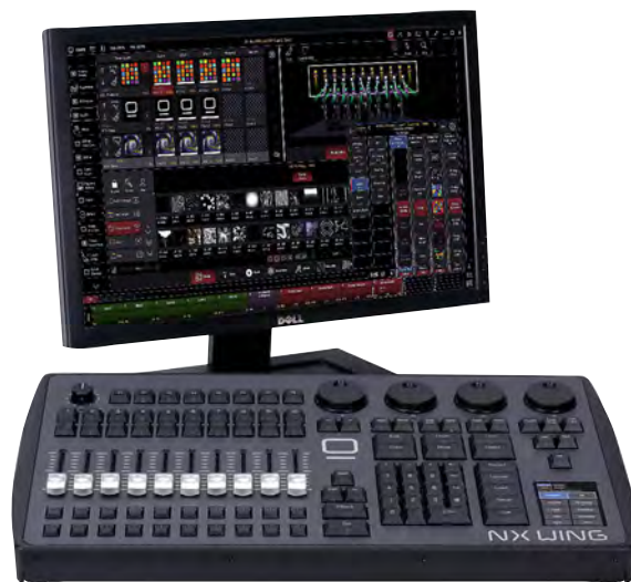
The NX Wing is the complementary USB control surface to Obsidian Control Systems' ONYX platform
