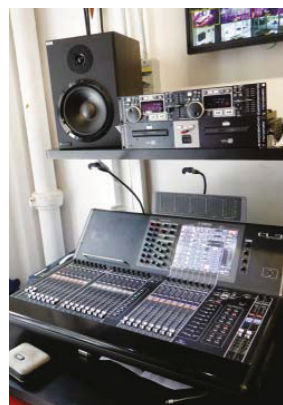
(Right): A Yamaha CL3 digital console can be controlled from an iPad via the Stagemix App
